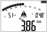
Use **SET/SEL** to display values of leakage current  $I_L$ .
