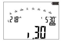
The value of leakage current I<sub>L</sub> measured in time t=5'30'. Symbol 1.30 indicates the selected time interval, in which the leakage current value was recorded.
