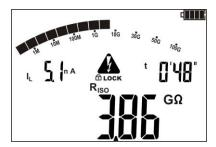
Use **SET/SEL** to display values of leakage current I<sub>L</sub>.
