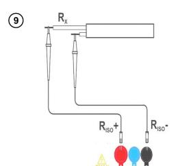
Connect test leads according to the drawing.
