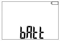
The battery pack is fully discharged, all measurements are blocked.
