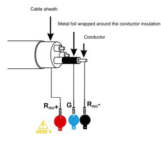
The same shall apply when measuring the resistance between two conductors of the cable, attaching to **G** terminal other conductors that do not take part in the measurement.
