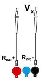
Connect the meter to a voltage source.
