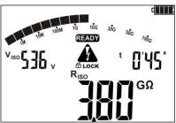
After the measurement is completed or stopped, read the result. The results of all completed measurements will be displayed (even when the measurement was interrupted/stopped e.g. after 60 sec.). When the meter switched into standby mode, the measurement result may be recalled by pressing **ENTER.**
