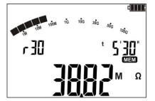
Resistance  $R_{\text{ISO}}$  value, measured in time t=5'30'. Symbol  $r\frac{11}{2}$  indicates the selected time interval, in which the resistance value was recorded.
